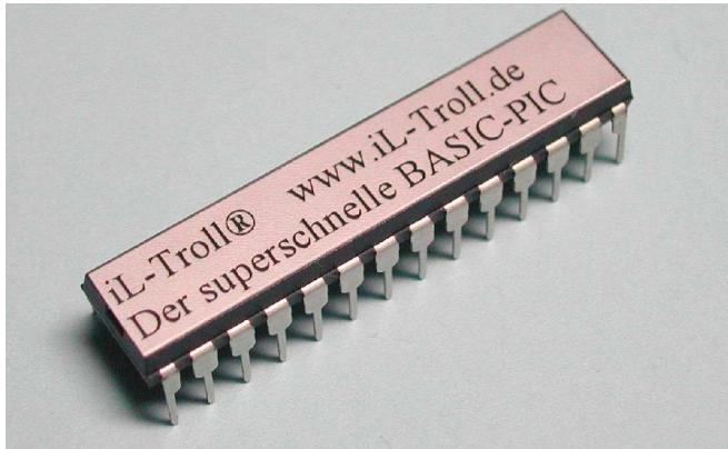
**iL-TROLL®** is a preprogrammed microcontroller. Its bios supports a simple download via RS232. For communication with a computer only 1 pin is needed. Only a small interface pcd is necessary for level shifting. Not only download but a comfortable program testing is available. This tiny bios (just 256 words of memory contains a remote debugger. Functions like SINGLE STEP, CONTINOUS MODE, BREAKPOINT and RESET. Watch and modify variables.
